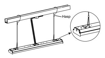
Step 1 : Mount cable to the luminaire. Tie the one end of cable to the beam, then insert into the hasp, adjust the cable to be desired height.
