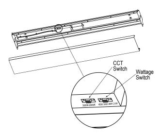
The end users may adjust the color temperature and lumen output respectively by the two DIP switch buttons integrated into the driver. DIP switches are accommodated with 4 and 5 options (left, middle and right), corresponding to 5 color temperatures and 4 powers respectively, which can perform the desired color temperature and lumen output combination.
