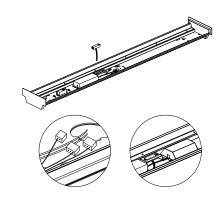
Step 1: Remove the lens and wiring connection cover box.(Figure 1)
