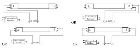
Voltage Input: AC120-277V 50/60Hz
