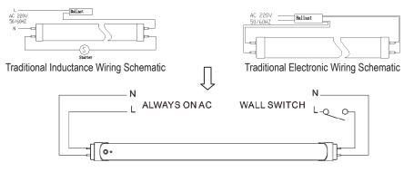
Led Tube Wiring Schematic
