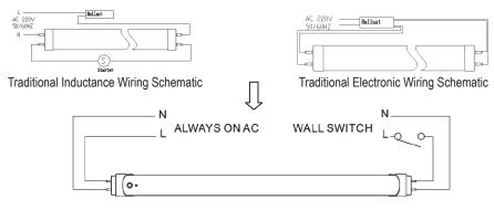
Led Tube Wiring Schematic
