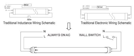
Led Tube Wiring Schematic
